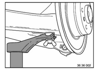
Apply balancing gauge on trailing arm as close as possible to wheel.
